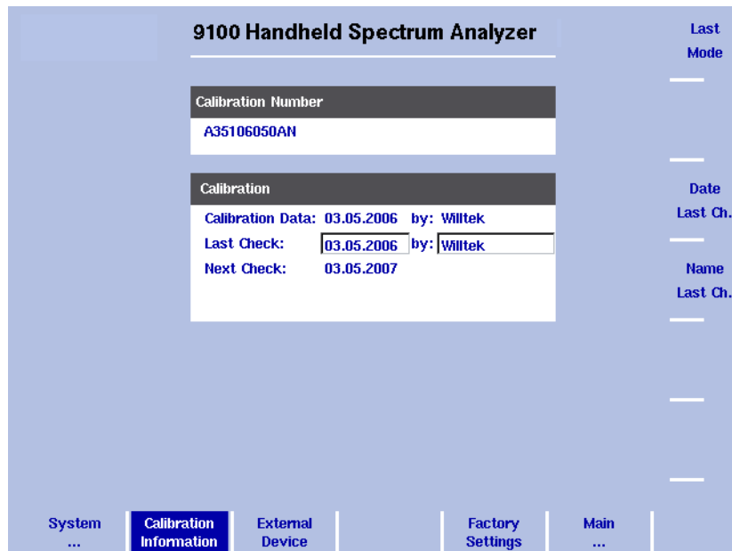
Figure 9 Calibration Information menu
